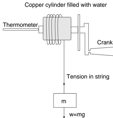
Figure 1: Sketch of apparatus used in this lab.
