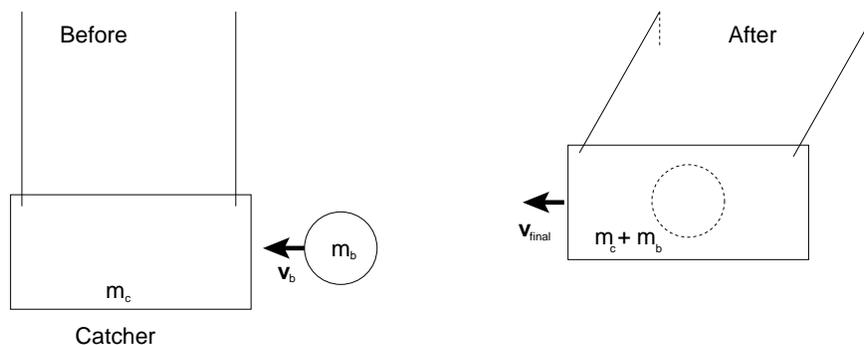
Let us first consider the first part of this motion, the collision of the moving ball with the stationary pendulum. After colliding, the ball is stuck in the pendulum and both are moving with the same velocity. We know this to be a perfectly inelastic collision which means that the kinetic energy in the system will not be conserved. The momentum of the system, however, will be conserved. Conservation of momentum may be applied assuming all motion is in the horizontal direction:
